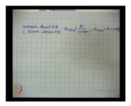
And finally, in the last configuration Current Shunt feedback which is also known as shunt series feedback the input impedance is reduced and this is a Zi FB equals to Zi 1 plus BA and the output impedance increases so, Z out FB is equal to Z0 1 plus BA so, this are the expression for the impedances the modified impedances for a amplifier circuit which incorporates negative feedback.
