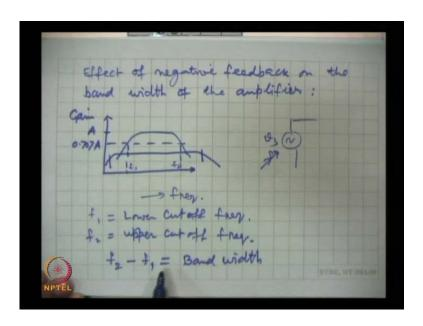
Now, we continue this a feedback a studies and we take the effect of a negative feedback and the band width of the amplifier, effect of negative feedback on the band width band width of the amplifier we study these thing yes, negative feedback enhances the band width first let us see what is band width. In general for any amplifier if we plot the game versus frequency response meaning that here this is the input signal and
