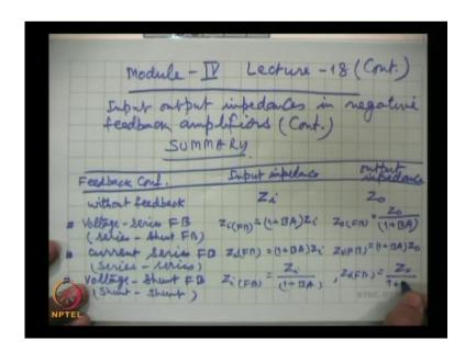
So, this is the summary for all the four configurations, this is the feedback configuration, this is input impedance, and this is the output impedance, input impedance and output impedance. Now without feedback this is input impedance is taken as Z i and the output impedance is taken as Z 0.
