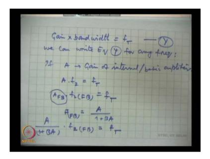
If gain increases band width false and the product will is still be equal to fT and if the gain of the this we can write for any frequency, we can write equation y for any frequency and for any frequency that gain will change and hence, the band width will also change making this constant.
