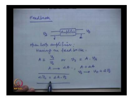
So, feedback in a amplifier, this is the amplifier, these are the two outputs and these are the inputs the signal is given here and the signal is the taken out here. Now, you know what is the purpose of amplifier? The purpose of amplifier is to amplify the signal without changing its characteristics except its magnitude. So in obviously, the output in a
