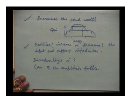
Further, it increases the band width for example, the gain frequency characteristics in general for in an amplifier are like this and this is called the band width. This bandwidth can be increased by incorporating the negative feedback.
