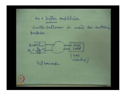
very low. So, the biggest application for this amplifier is as a buffer buffer amplifier by buffer we mean a intermediate between two states. So, it is used for matching purposes this emitter follower emitter follower is used for matching purposes what is to be matched I will just call for matching purposes. So, it is used as a buffer amplifier we have suppose because in the actual system there are several stages.
