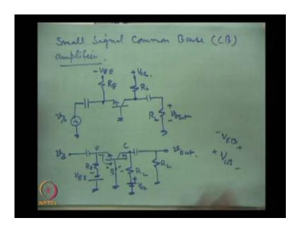
a small signal common base amplifier. In this circuit the input is connected input signal, signal to be amplified is connected to the emitter and it is connected through a capacitor.
