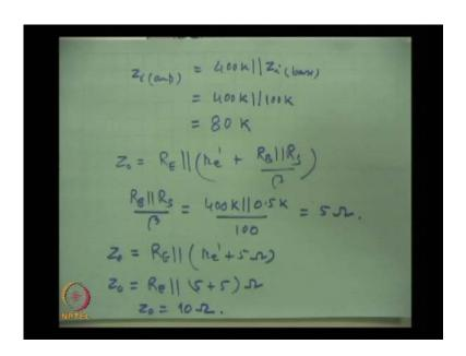
So, Z i amplifier is equal to 400 k and parallel with Z in base this is 400 k in parallel with 100 k and when you again solve it it will come out to 80 k. So, the input impedance of the amplifier is quite high. Now the output impedance Z 0 we arrived at the expression R E in parallel with r e prime plus R B in parallel with R S by beta this is what we arrived at. We talked about this and now R B in parallel with R S beta this is 400 k into 0.5 k
