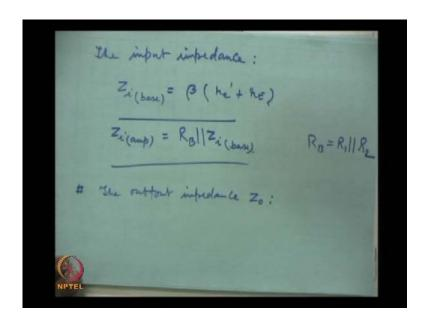
the input impedance the input impedance. If you look this circuit which the ac equivalent circuit of the emitter follower here the difference between this circuit and common emitter circuit was simply that we take the output from the collector, but R E was still there.
