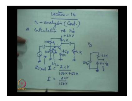
For example, we remember that this was the common emitter circuit and when we see here this is Z in i base z in i base and when we take the biasing resistance into account.
