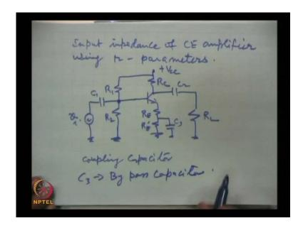
Input impedance using r parameters, the circuit under consideration I redraw(No audio from 13:50 to 14:19) plus V C C this is the coupling capacitor, this is the load across which we will measure the output voltage and here, this is the input signal and this is resistance R 1, this is R 2, this is R C and so on and these capacitors - these are coupling capacitors and this is called bypass. So remember these names coupling capacitor and this is C 3 is bypass capacitor.
