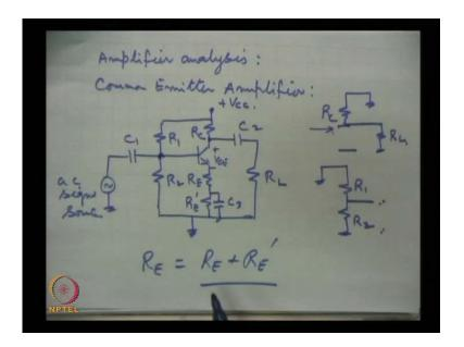
Now, let us take this as an example, we were here that actually a best compromise between stability and high voltage gain can be obtained by breaking the resistance R E into two resistances R E plus R E prime. Now, so these are the two resistances, this may be small resistance as compared to this, but not small enough to to in comparison with the dynamic emitter resistance. So for example, it may be 200, this may be 800 and so
