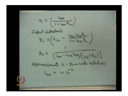
And the current gain for the common emitter amplifier is h f e by 1 plus h o e, R L this is the expression exact expression for the current gain of the common emitter amplifier. We have input impedance input impedance and that is for c amplifier Z i is equal to h i e minus h r e, h f e R L by 1 plus h o e R L and finally, the output impedance Z 0 for common emitter amplifier 1 by h o e minus h r e and h f e divided by h i e plus R S.
