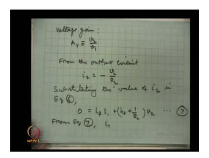
So, first we derive a expression for voltage gain. We now get an expression for voltage gain and which as I said is equal to A V as the ratio of this two voltages. Now from the as I said we will have manipulate this so, that we get this ratio to and this should not involve any unknown parameter.
