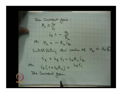
gain, current gain will be it is written as A i and this will be the ratio of i 2 over i 1. So, again we have to clear with the equation we have to manipulate the equations in such a way that this ratio is equal to the terms and which each parameter is known that we will see.
