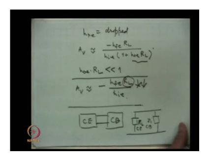
We drop h r e dropped then we get the approximate relation and again I repeat approximate means within few percent which is acceptable and most of the applications in electronics. So, a accuracy does not suffer significantly and this is equal to minus h f e
