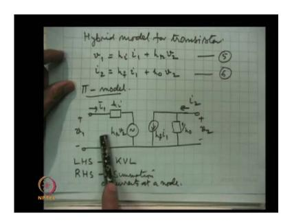
So, in this pi model which we have arrived yet, now the transistor will be replaced by this and we have we have to add this part and this part to the pi model. So, what we get is this.
