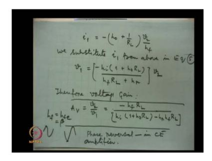
i 1 is equal to minus h o plus 1 by R L, v 2 by h f. We substitute for i 1 we substitute i 1 from above two equations 5 this is the equation. So, i 1 because here we want the ratio of v 2 by v 1 we we are finding the voltage gain which is the ratio v 2 by v 1. Now here i 1 should be replaced by the known parameters and here there are mostly the known in fact this will be taken care of automatically.
