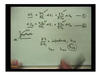
And this is d V 1 the total change in V 1, this depends on (No audio from 14:21 to 14:42) this term the first term, this is the rate of change of V 1 on I 1; and if I 1 changes by d I 1 then this gives the total change in V 1 as a result of change d I 1 change in the current. And this term is the change in V 1, because of V 2, when so this is the rate and this is the total change in V 2 and hence, this is the total dependence of V 1 on I 1 and V 2.
