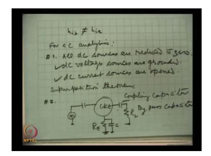
That h i b, this represents the input impedance in the case of the common base and this is certainly not equal to h i e that means the hybrid parameters, the same parameter in different configurations common base, common emitter and common collector, they are different. And we will see that, how we can get the value of the parameter in other configuration like common base or common collector, because the manufacturers specify
