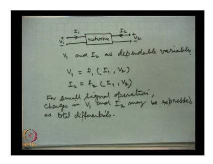
The network is or this is just the transistor and these are this is I 1, this is V 1 and this is I 2 and plus minus V 2. The parameters can be defined by taking out of these four quantities, the two currents and two voltages, two are taken as independent and two are taken dependent. So, we can write the fundamental relation for dependent variables, we take V 1 and I 2 as dependable variables.
