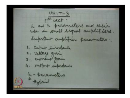
These parameters are (No audio from 03:03 to 03:15) important amplifier parameters, one is the input impedance input impedance you know that, resistance and impedance they are they may differ at high frequencies; when the frequencies are small, then resistance and impedance they they are very close to each other. And so, we may call input resistance or input impedance, but it is better to call input impedance, because frequency we are not yet defining.
