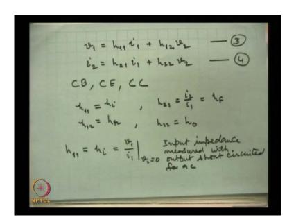
And then, we can write these equations 1 and 2 like this v 1 equal to h 1 1 i 1 plus h 1 2 v 2; and i 2 is equal to h 2 1 i 1 plus h 2 2 v 2, this we call equation 3 and this we call equation 4. Now, these equations are applicable to all the configurations of the amplifiers, whether it is common base, common emitter or common collector, these equations are valid. And in fact, the whole analysis which we are trying to study, they are applicable to all these circuits.
