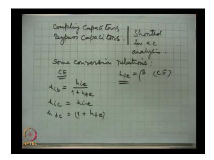
These are coupling capacitors and bypass capacitors. So, AC analysis needs and this is the requirement as the first requirement was that, the DC sources have to be reduced to 0. Similarly, these capacitors are all taken as shorted capacitors these are shorted for AC analysis. Now, I give you first some conversion relations some conversion relations that is I said that, common emitter is most widely used amplifier.
