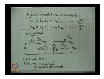
Now, the hybrid model hybrid h model, hybrid model for transistor for example, the two equations are, v 1 this is h i i 1 plus h r v 2; and similarly, i 2 is equal to h f i 1 plus h o v 2. These equations we will be now using and let us call these equations, and and from
