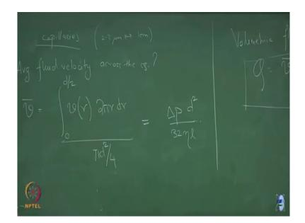
So, what is the average fluid velocity across the cross section cross section? Which means that I need to take the average. So, v average across this cross section is this v of r into 2 pi rdr right r growing from 0 to d by 2 divided by pi r square. So, pi d square by 4, ok. So, this is right this is the average fluid velocity over the cross section v r 2 pi rdr divided by the cross sectional area.
