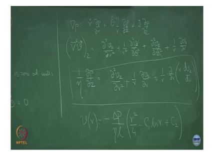
So, the obvious choice is to work in cylindrical coordinates, right because the problem is cylindrical symmetry. So, the gradient of p in cylindrical coordinates is r hat del p del r plus theta hat 1 by r del p del theta plus z hat del p del z. And, the Laplacian the z component of the Laplacian is del 2 v z del r 2 plus 1 by r square del 2 v z del theta 2 plus del 2 v z del z 2 plus 1 by r del v z del r.
