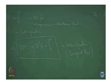
So, this is the full Navier-Stokes. So, this is Navier-Stokes remember for an incompressible fluid, for an incompressible fluid otherwise we will have another second derivative term and Newtonian fluid, right. So, one of the limits that is one of the limits of this equation is when you have a fluid with no viscosity.
