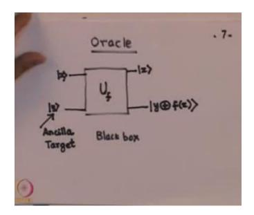
So this is Ancilla also that target bit, this is where the output will be there. Now this  $U_f$  function takes X at the input computes effects and output is here leaving the input the same. So this is unchanged and here what you get is the EXOR of y with the effects. So this is the way an oracle is represent, now you notice that supposing you said y=0 which means this is zero plus effects which by definition effects.
