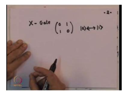
X-gate is simply given by 0110 is standard Pauli matrix and its job is to take the  $|0\rangle \rightarrow |1\rangle$  and vice versa. So this is basically equivalent to a classical not gate, like X-gate we have Z-gate which changes the sign of the component 1 and also we have a Y-gate which is given by a matrix very similar to the Pauli Y-matrix, I will write it down.
