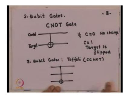
The most significant is what we called as the control NOT gate or CNOT gate if you recall what CNOT gate is that a CNOT gate basically has a control and a target. So the, its representation and circuit is like this. So if control = 0, target remains target, no change if control = 1 the target bit is flipped that is 0 becomes 1 and 1 becomes 0. So if C = 1 target if flipped, we also talked about a few 3 qubit gates.
