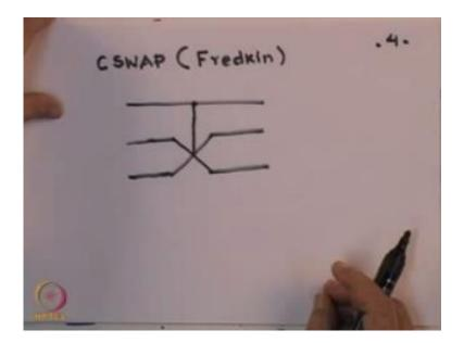
CSWAP which is also called a Fredkin gate, so basically a Fredkin gate again has a control, but there are targets on which it will act and so this is essentially flip the targets. So this is your control it will flip the target if the control bit happens to be equal to one. So these where the elementary gates which we talked about and what we are going to do today is to talk about quantum circuits.
