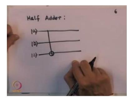
So let us look at how does a half adder circuit work. so this is a and this is b and what I do is I set this third one to 0 remember each one of them a single cubit so a and b can take value, you know 0 or 1 each. Now I start with the circuit which is a CCNOT gate so notice remember what is the CCNOT gate.
