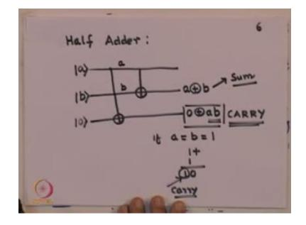
So this is the way we implement half adder you can do some practice on this type of a implementation of classical circuits, for example try what is the full adder and thinks like that. Now there is another important component of a quantum circuit before we write down a full fledged quantum circuit we need to understand this a little bit and this is what is known as a oracle not to be confuse with the corporations having the same name.
