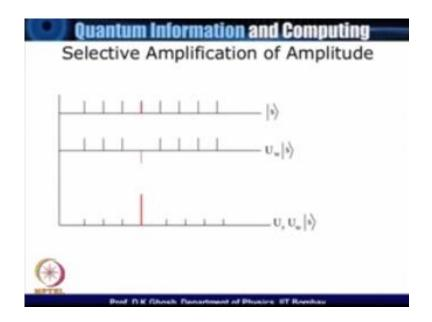
Review to calculate and let see that after one Grover iteration the amplitude becomes five times the amplitude of the inter given that the end of state.
