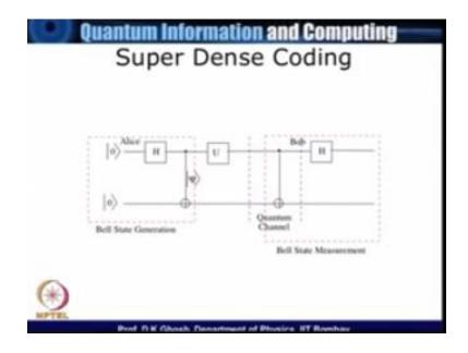
So this is a schematics of the type of circuit that we have, the left-hand part of the circuit which is enclosed in that red dotted rectangle is really not a part of our process because that is simply telling you the, how a bell state is generated actually. So you start with the two states 00 and then you apply a Hadamard followed by a CNOT that is the way to generate the bell state. So therefore, the left-hand side part is simply a bell state generation.
