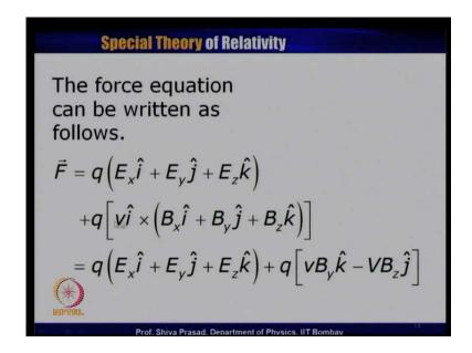
So, this is what I have written here v multiplied by B z i cross k is minus j which brings this minus sign and this is j. So, this is what I have written here. Now like before I will pick up the x component of the force y component of the force and z component of the force. So, these will be the force which we experienced by the particle in S frame of reference. If the electric field was E and the magnetic field was B both at this moment of time, I do not know what is E and B.
