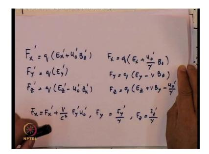
equations in this particular paper because I am going to use this things F x prime is equal to q E x prime plus u naught prime B z prime F y prime is equal to q E y prime f z prime is equal to q E z prime minus u naught prime B x prime these equations will see later.
