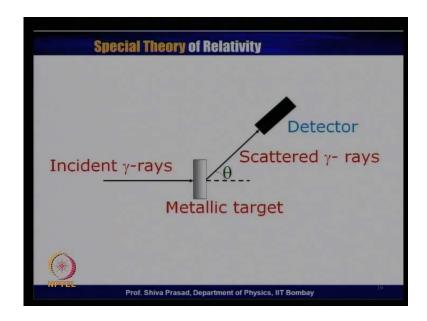
We have a metallic target. There is an incident gamma ray, which comes and hits here and we have a detector, which detects gamma rays. It is possible to obtain detectors, which can detect and which can count, which can tell how many photons have come at a particular angle.
