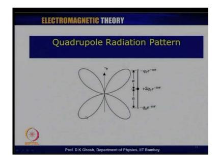
The quadruple radiation pattern shows the maximum at angle equal to pi by 4 and this is the way the quadruple moment looks like this is something, which you will you will do well to take it as an exercise. So, this is basically what we want to talk about in the radiation basically talking about how the power you know is transported? The radiation zone is 1 over r and how much is the power which is sent from the the transmitting antenna, which is later on received by a receiver antenna.
