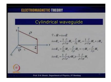
So, let us let us look at the geometry of this, so this I recall for you my cylindrical geometry I have x axis here, y axis there, so it is basically a polar coordinate, given by a rho and phi and of course, the z axis the z direction remains exactly the same. So, rho and phi are along the two dimensional cross circular cross section, and z is of course, along the right direction. So, what we will now do is this, we will write down the Maxwell's equations in the cylindrical geometry.
