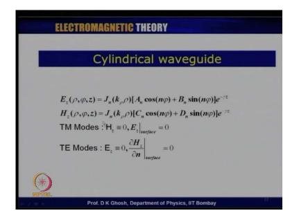
So, therefore, my solution for either E z or H z depend upon which mode you want, will be J n, n is an integer, a function of k rho rho, times this sin cosine which came as a solution on the phi equation, times E to the power minus gamma z. If I am looking at T E mode my E z is equal to 0, but the normal component of the magnetic field d H z by d n on the surface will be equal to 0; if I am looking for T M mode H z equal to 0, E z on the surface will be 0.
