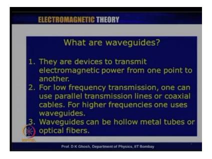
So, as we have pointed out a typical waveguide consists of a hallow metal tube, which is one of the ways of having transferring power. The other more common place today for example, optical fibers, which are widely used today to carry signals, the light signals for example, from one place to another.
