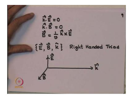
What I have got is, k dot E is equal to 0, k dot B is equal to 0, B is equal to 1 over velocity times k cross E. What is the import of these equations? These tells me that E and B are perpendicular to k; and this tells me that E and B themselves are perpendicular to each other. So, it means that the electric field, the magnetic field and the propagation vector k, they form a triad, a right angle triad; they are mutually orthogonal and they form a right handed triad.
