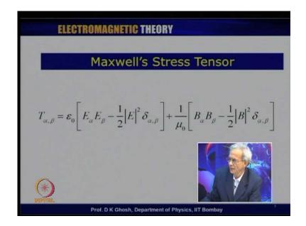
This was our expression for the Maxwell stress tensor, in terms of which we had defined the momentum density of the electromagnetic waves. Basically, it has 2 terms- one is for, from electric field, the other is from the magnetic field; and the expression is fairly simple. (Refer Slide Time: 02:46)
