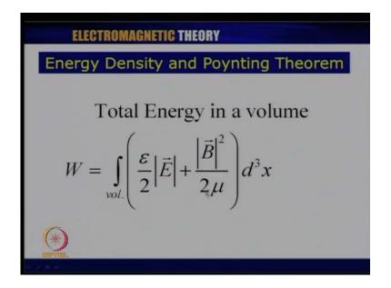
The total energy in a given volume del E is given by the volume integral of this quantity so that is the total energy in a given value.
