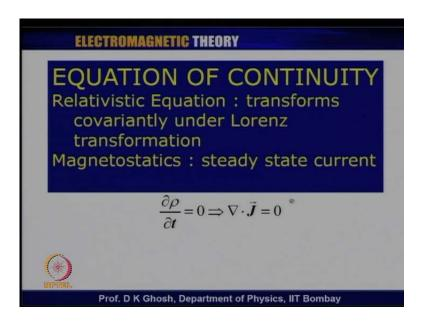
Since, we will be interested in, primarily magnetostatics, namely my currents are steady. So, therefore, I must have d rho by d t equal to 0, because there is no accumulation of charge in the volume. And as a result, the corresponding equation then becomes del dot of j equal to 0. So, this is the steady state form of the equation of continuity.
