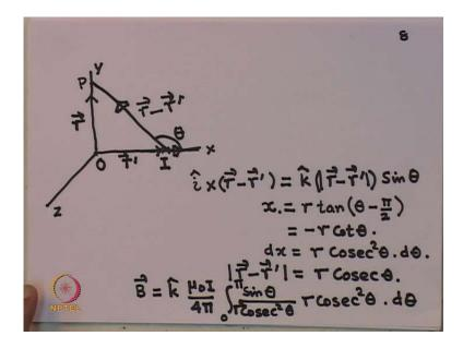
So, if I use Biot Sarvat's law, let us look at, how does it work? So, let me, let me define the x, y, z axis in the same way; this is my x axis, this is my y axis, and the z axis is out of the plane of the paper. Now, my, I will take the wire in the direction of x axis, and the point at which I am interested in calculating the magnetic field to be at, on the y axis; remember that I can always do it, because I have an infinite wire.
