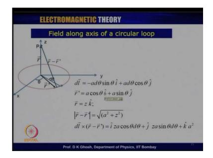
So, let us refer to this picture here. So, I have taken my circle which is in red, in the x y plane. So, this is x axis, this is y axis, and z axis is along the axis of the circle that is perpendicular to the plane of the circle passing through its centre. So, remember that, what I am going to do, I need my, to apply Biot Sarvat's law. So, I first need an expression for d l, remember I d l cross r minus r prime. So, let us look at the vector relationship first.
