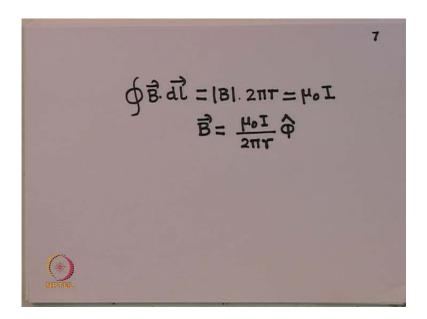
So, in that case, what I can do is, I can calculate what is the integral of B dot d l, by taking a circle of radius r. Since, B is the azimuthal, and the circle that I take is also in the same direction, B dot d l is same as magnitude of B times magnitude of d l; and then the integration, since magnitude of B is the same and the integration over d l will be matching dot 2 pi times r; and that must be equal to mu 0 times the current that is flowing through.
