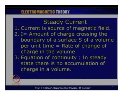
So, in other words, this is, supposing I take a volume, which is let us say, defined by a boundary S. The rate, so if certain amount of charges flow into the volume, the amount of charge in that volume will increase. Now, in steady magnetic phenomena or in a steady state phenomena, I do not expect an accumulation of charge; and this gives rise to what is known as the equation of continuity. Now let us look at, what is equation continuity?
