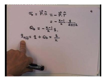
Now the surface charge density we have seen is p dot n. You remember that I have a sphere but then the dielectric medium is inside the sphere and the surface normal is not along outward radial but along inward radial. So therefore, it is minus p dot r and this is equal to minus, well, p dot unit vector r. So therefore, it is kappa minus 1 divided by kappa times q by 4 pi r square. So, this dielectric sphere that I have got with a charge
