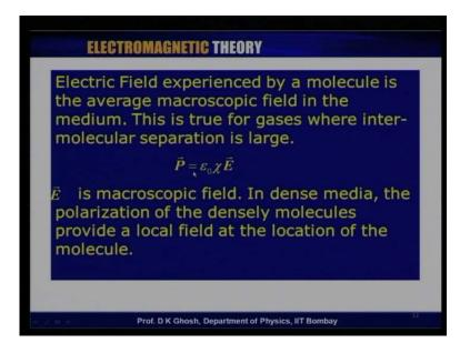
Remember that the polarization can be written as epsilon 0 chi E which is the susceptibility times the electric field and E is the microscopic filed. Now if you consider however, a dense medium however the molecules are packed close. Then if you consider a particular molecule, then the electrons in the vicinity of that molecule, they will be polarized of course and they are responsible for producing what we can call as a local field at the location of the molecule which we are considering.
