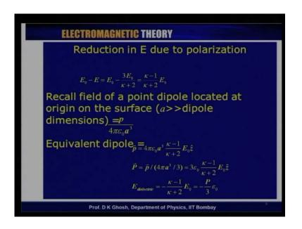
But when we calculated the electric field we found that it is given by E which was minus 3 E 0 by kappa plus two.
