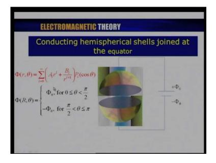
Let me give you another example. In this case, I have two conducting hemispheres. I have just pictorially separated them. The northern hemisphere is connected to a potential phi 0 and while the southern hemisphere is connected to a potential minus phi 0. Now, what we are interested in is, what is the potential inside the sphere? Now, look at this. I have got phi 0, the general expression for phi R theta is what I started with last time.
