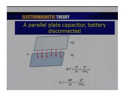
So, for example, let us consider a parallel plate capacitor from which the battery has been disconnected. So, what I will assume is that the initially the two capacitors are charged to plus Q and minus Q and let me assume that one of the plates is fixed. Let us say by bolt it is not allowed to move the other one is allowed to move.
