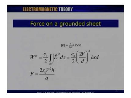
Now, if I look at that then in the region where this grounded sheet has entered and I have put it right at the centre let us say. Now, an electric field has been established and this electric field has a Magnitude equal to V divided by d by 2 because d by 2 is the distance between the grounded sheet and either of the plates which is equal to 2 V by d. Now, the electrostatic energy of this situation is epsilon 0 by 2.
