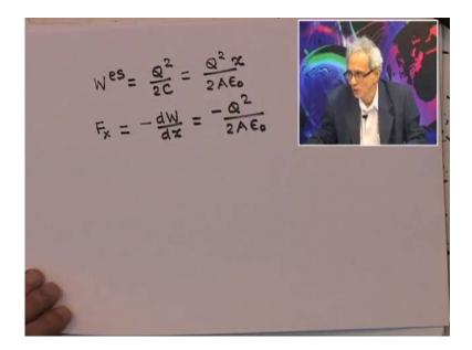
Now, I know that the electrostatic energy of the problem is W e s and that is equal to Q square by 2 C. Now, the capacitance expression is known to be so it is Q square divided by 2 a epsilon by 0 times x, where x is the instantaneous distance between the two plates.
