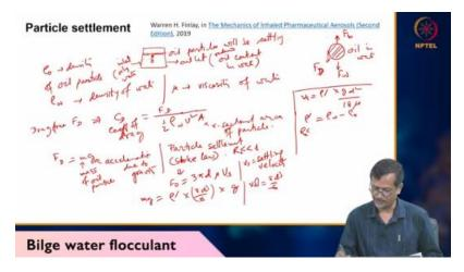
or in simplified form we can derive like this Vs equals root over 4 g rho w minus rho oil because rho dash we have written rho w minus rho oil d d oil square 3 c d rho. CD equals 24 by RE. This is laminar flow. RE becoming D oil U oil rho by mu. UVS equals G D square rho water minus rho oil by 18 mu.
