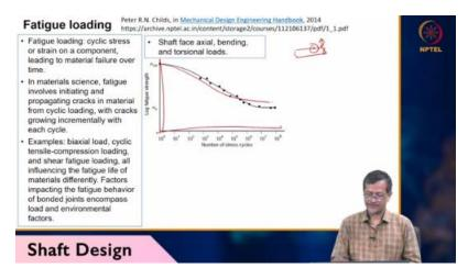
This occurs due to irregularities in the object's geometry or material, such as holes, grooves, notches, disrupting stress flows. A non-dimensional factor called stress concentration factor is used. For example, you have one shaft, and you have a small crack here. What is happening? The total area is here, A.
