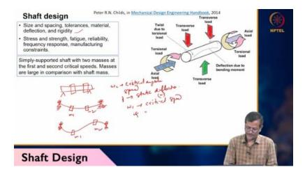
Soft will have its own weight, so it will have sagging tendency. It will have some pulleys or gears mechanism, so that soft will try to bend or it will shear. So, we will just try to discuss how to design using all these forces. So, ASME document, they are saying like 50 to 9% of all mechanical failures are due to fatigue failure. 50 to 90 percent of all mechanical failure of shaft mechanical failure of shaft is fatigue failure now we have seen sharp material sharp material
