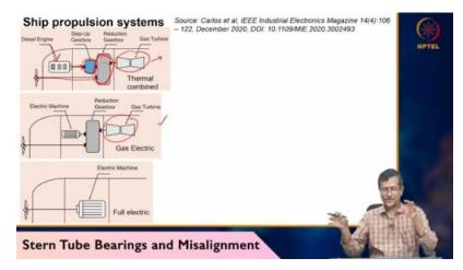
Maneuvering will be easier. So, DC or AC motor or propulsion system motor runs propeller. A generator and prime mover assembly produce electricity. Traditionally employed in smaller vessel, efforts are going to use larger cargo vessel. used in tugboats and trawlers dredges dynamic positioning vessel cable line shapes icebreakers many applications are there so i already told the shaft alignment is a big issue here one example is given you can see this picture if shaft is aligned properly
