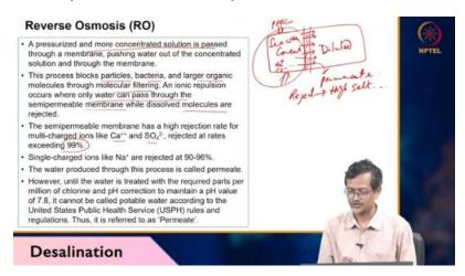
You are collecting pure water here. you are collecting pure water here. And your reject is going here, the rejected water. So, it is flowing through several layers of your membrane, then you are getting water. So, RO membranes commonly exhibit removal efficiency ranging 90% to 99% for contaminants like total dissolved solid.
