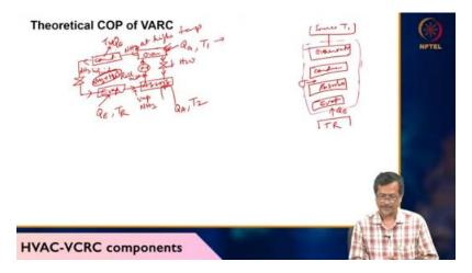
greater than equals zero okay so minus qg by t1 plus qe plus qg t2 minus qe by tr greater than equals zero so or qg by t1 plus qg by t2 QG by T2 plus QE by T1 minus QE by TR greater than equals 0. from there we get T2 minus TR. T2 TR QE less than equals T1 minus T2 T1 T2 QG so QE by QG QE by QG less than equals T1 minus T2 T2 minus TR TR by T1 so COP equals QE by QG less than equals T1 minus T2 by T2 minus TR TR by T1 so maximum COP equals T1 minus T2 T2 minus TR
