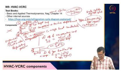
And eta volume, already we defined volumetric efficiency. In this way, we can calculate volume of gas handled by a reciprocating compressor, which is having multiple cylinders, maybe, or one cylinder also possible, because based on value of n, we can calculate. And whenever you are calculating, you have to see the units. Units must be balanced, left side or right side. Okay, these topics are taken from P.K. Nag book.
