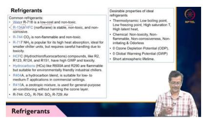
So, water, you should remember the name also like R7, R means refrigerant. R means refrigerant and 718 some nomenclature is there. So we will discuss later. So R134A, R744, carbon dioxide also can be there, ammonia can be there, hydrochlorofluorocarbons, HCFCs also will have refrigeration properties, hydrocarbons like R600A, so several refrigerants are there then ample names are there but we normally for you our case will be studying
