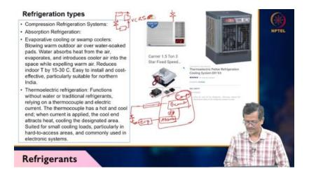
Air will be entering here. Then air will be going out from here. And it will be soaked with water. When you are soaking, air is going through the soaked cotton or the sieve. So the air will get lots of moisture.
