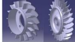
3D models of turbine vane and rotor Nicora et al. Axial Turbine Performance Estimation During Dynamic Operations. Int. J. Aeronaut. Space Sci. 22, 359–365 (2021). https://doi.org/10.1007/s42405-020-00312-4
