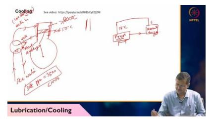
So, my marine engine is here. So, marine engine will be getting cooled because of this circulation of fresh water, but this heat is taken by seawater. So, seawater will be passing through this heat exchanger that will be reducing my fresh water temperature. This is simple line diagram. Any drawing you can do and you can explain how things are working.
