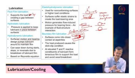
So, in sliding operation, the energy dissipation must be there. So, if energy is not getting dissipated, so heat will be accumulated. In many systems, if heat is getting accumulated, it will be reaching up to melting point of the two surfaces, one surface or both surfaces. So, in that case, local galling operation or local welding operation will be happening. What is happening like this?
