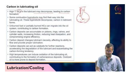
Oil means lubricating oil system contributing carbon formation. Carbon deposits can accumulate on piston, ring, valve, cylinder valve, increasing friction, reducing heat dissipation and compromising engine efficiency. So, so many negative effects are there. So, you have to change your lubricating oil from your bike regularly. Carbon deposits accumulate
