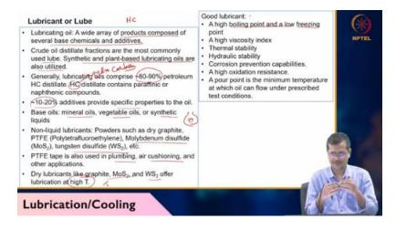
Thermal stability, so it should be stable in thermal. Hydraulic stability should be there. Corrosion prevention capability, so you have to add some additives so that it should help not to corrode the system. High oxidation resistance must be there. A pore point is the minimum temperature at which the oil can flow under pressure.
