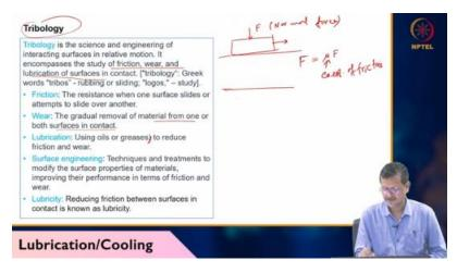
Lubricant or lube, so sometimes they say lube or lubricant. Lubricating oil or if you go to any petrol pump they will say engine oil. So oil normally in scientific term we say oil means any high viscous fluid, petrol, diesel also that is oil. But petrol pump those people will be assuming oil means lubricating oil. Lubricating oil is a wide array of products composed of several base chemical and additives.
