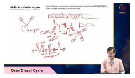
so in that case you need multiple cylinders so that will be smoothing the power and your flywheel requirement will be lower so flywheel means heavy mass you are carrying unnecessarily right heavy machine truck is there so instead of carrying the heavy mass you make multiple cylinder you get total power higher okay this is done. What is next topic? Terminology. Okay, so different terminology we will be using when we will be solving problems for IC engines.
