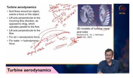
So, vortex creation means fluid is trying to touch, but it is unable to touch. So, what will happen? It will not get proper lift. So, when proper lift is not there, then there can be destruction or low torque you can get. And airflow gives maximum lift in a given air speed is limited by its boundary layer separation.
