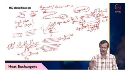
outside lots of fins will be there so that you are increasing surface area okay you are increasing surface area and you are increasing heat transfer rate so this is internal fin this is external fin okay and this pipe arrangement inside your heat exchanger also may be different for example this may be one piping arrangement central one like this okay so how to optimize it so inside pipe when fluid is flowing you are trying to create turbulence so
