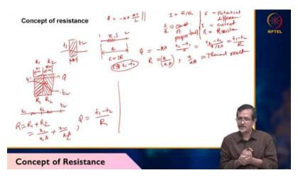
Q heat, same heat will be going out and R1 resistance is here, R2 resistance is here, temperature T1, temperature T2 and this distance is x. So, formula becomes R1 by R1 plus 1 by R2. So, r1 equals x by k1 a1, r2 equals x k2 a2. And if I have another slab also, I can write like this. So, if I have three slabs, so in that case, I can write like this R3 equals X by K3 A3. So, I have to make difference in hatching line also, because three different metal I am assuming.
