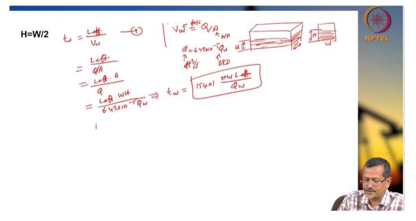
So the formula is 1.78 into 10 to the power minus 6 del SG dm square by V W Q by A. What is A? A will be this diameter D so pi by 4 diameter square and we are counting degrees140. So then V W becomes 6.49 10 to the power minus 5 W W divided by pi by 4 D square divided by 140. If we solve it this will be giving D square equals 6 6 9 1 F into mu del SG dm square.
