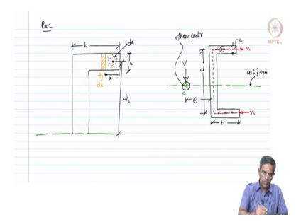
So, example 2. We will take up a channel section. We know the shear flow this is going to be. So, this is I calls  $V_1$ , I call this as  $V_2$  and we also know that this section has an axis of symmetry.
