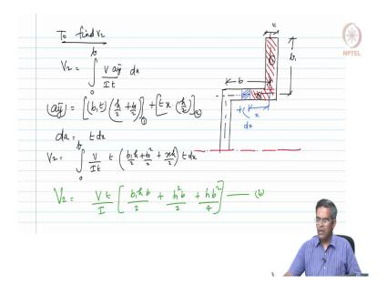
This may line of symmetry. We know this is  $b_1$ . I am marking the center line. We know this is  $b_1$  and the thickness is t uniform. I will cut the strip here at a distance x from here and let the thickness be dx.
