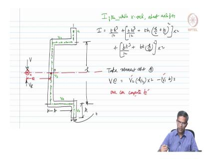
So, we want to find the moment of inertia of the whole cross section about axis of symmetry. So, let us do that.
