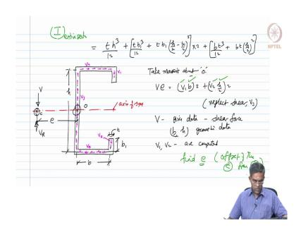
$$I_{entire\ section} = \frac{th^{3}}{12} + \left[ \frac{tb_{1}^{3}}{12} + tb_{1} \left( \frac{h}{2} - \frac{b_{1}}{2} \right)^{2} \right] \times 2 + \left[ \frac{bt^{3}}{12} + bt \left( \frac{h}{2} \right)^{2} \right]$$
