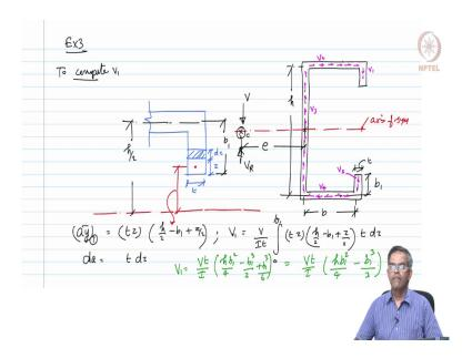
We will call this example 3. We say it is a very common section being used in marine structures a thin section having uniform thickness. So, let us say the dimensions are marked as shown in the figure this is b.
