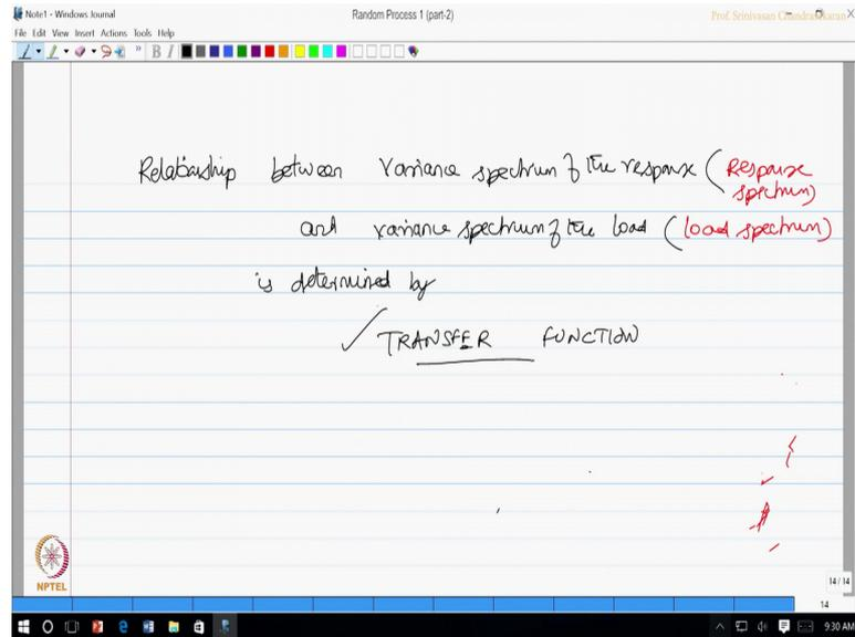
Therefore, the relationship between the variance spectrum of the response which we call as response spectrum and variance spectrum of the load which we call as load spectrum is determined by the transfer function. So, our job now is to determine or derive this transfer function which actually connects the response spectrum to the load spectrum.
