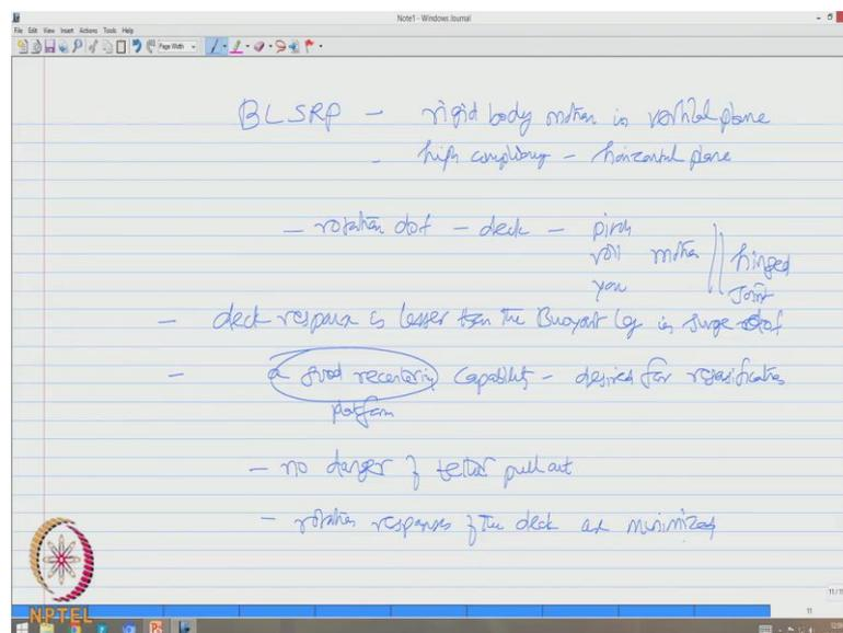
So friends, BSLRP show a rigid body motion in vertical plane and high compliancy in horizontal plane. So, the primary objective was to reduce the rotational degrees in the deck in terms of pitch, roll, and yaw motion which is now achieved by placing a hinged joint between the platform leg and the deck.
