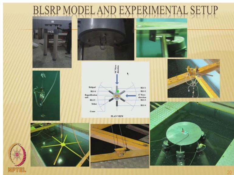
These are some of the elements of the platform which has been fabricated for experimental investigation. These are the buoyant legs, these are the hinged joints or the ball joints is a hook at the bottom of the buoyant leg which is being used to do connection of the tendon to the buoyant leg and the sea bed; that is a typical figure of the
