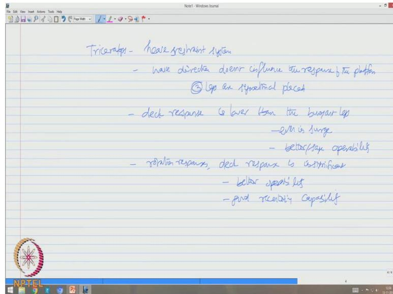
Therefore, one can say that triceratops have heave restraint system, because of this wave direction does not influence the response of the platform provided three legs are symmetrical placed. We also saw deck response is lower than the buoyant legs even in surge degree ensuring a better and safe operability. In the case of rotational responses, deck response is insignificant ensuring better operability and a good recentering capability.
