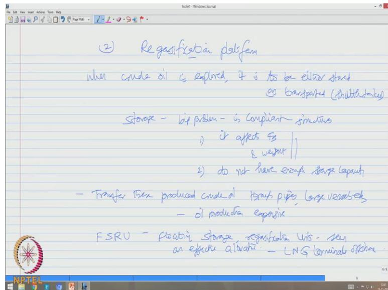
The next system what we will see now is regasification platform. We know that when the crude oil is explored from the drilling or the escalated platform; when crude oil is explored it is to be either stored or transported using a shuttle tanker. Storage is a big problem in company structures because it affects buoyancy, it also affects the weight, and therefore the platform stability may be challenged. The second issue is these platforms do not have enough storage capacity also.
