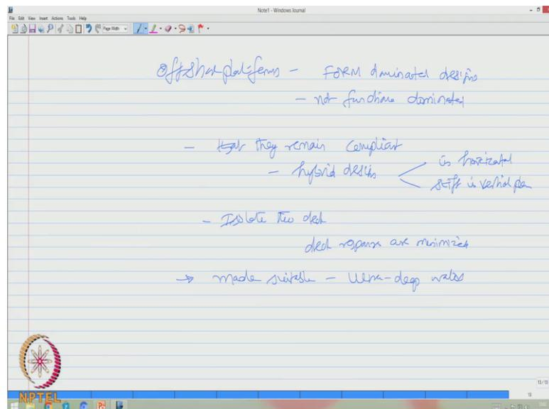
So, now we understand that offshore platforms are form dominated designs, they are usually not function dominated. It is preferred that they remain compliant, but we need a hybrid design. In sense compliant in horizontal plane, but stiff in vertical plane. We also saw when we isolate the deck responses are minimize. Therefore, this platform can be made suitable for ultra deep waters where the forces are much higher compared to the deep and shallow waters.
