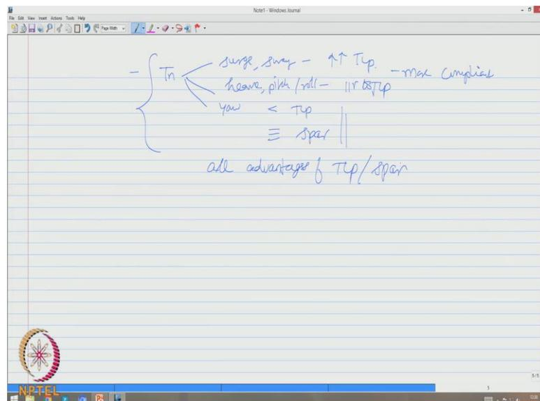
Natural periods in surge, sway are slightly higher compared to TLP. Making it more compliant in heave pitch and roll they are similar to TLP. In yaw it is slightly lesser compared to TLP, but more or less similar to that of a spar. So, the system derives all advantages of TLP under spar platform.
