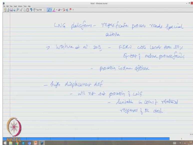
So, LNG platform which houses regasification also needs special attention. So, by Wenhua in 2013 it is seen that FSRUs cost lesser than 50 percent of that of onshore processing facility. So, it is expected that processing is done offshore. The conventional platforms what we have today like TLP, spar, etcetera have very high displacement degrees of freedom. They will not suit processing of LNG, because LNG terminals require a very high limitation in terms of rotational responses of the deck.
