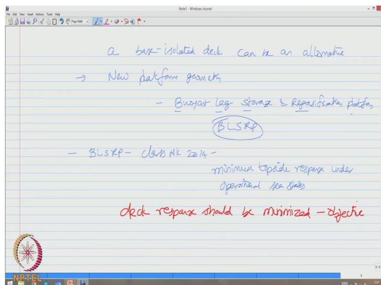
So, a base isolated deck can be an alternative. So, a new platform is conceived, a new platform geometry is conceived which we are going to discuss now that is called Buoyant Leg Storage and Regasification platform, so we say BLSRP. The foremost condition of a BLSRP as per class NK 2014 is it should have very minimum topside response under operational sea states. So, the condition here is deck response should be minimized, that is what the goal; that is the objective.
