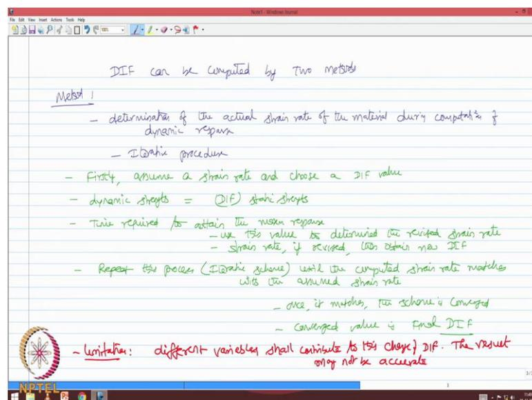
There are two methods available in the literature based on which DIF can be computed. The dynamic increase factor can be computed by two methods, let us see method one - the method one demands determination of the actual strain rate of the material during computation of dynamic response, this is an iterative procedure. Let us see what are the steps involved in this procedure, first assume a strain rate and choose a DIF value.
