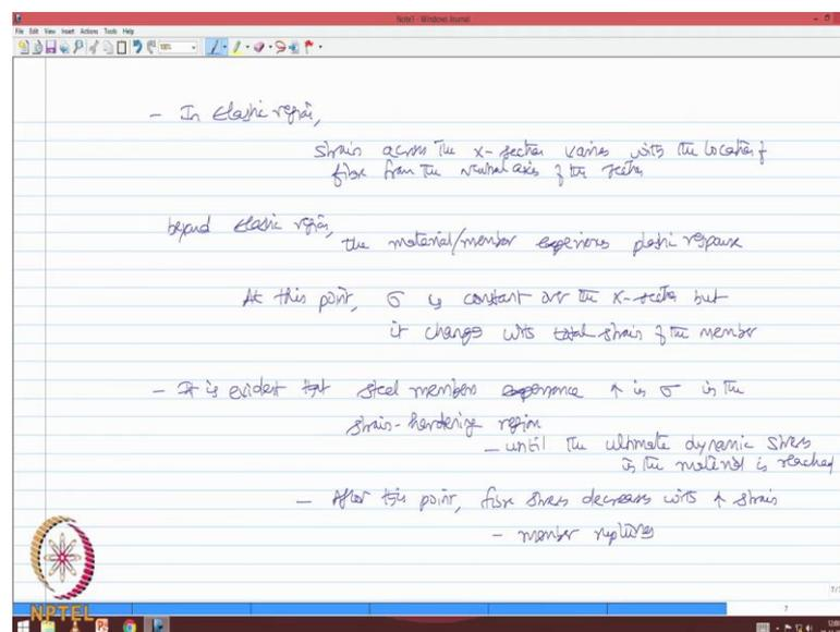
Of course in elastic region, strain across the cross section varies with the location of the fibre from the neutral axis of the section. Now beyond elastic region, the material and the member experiences plastic response. At this point, stress is constant over the cross section but it changes with the total strain of the member, so the variation is now shifted from the cross section to the member dimensions.
