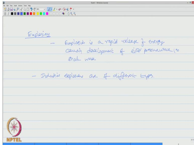
Let us ask a question more in detail about explosions. We all said already that explosion is a rapid release of energy causing development of either a pressure wave or a shock wave. Industrial explosions are of different types; let us see one by one. The first one in the list is CVCE what we called confined vapor cloud explosion.
