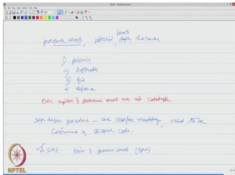
If you look at the pressure vessels which are one of the important candidates of explosion, there are different potential health safety hazards; one could be poisoning, two could be suffocation, three could be fire and fourth can be explosion.
