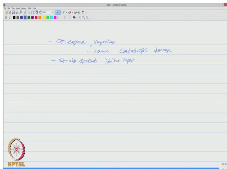
On release it expands vaporizes and therefore, causes catastrophic damage to the vessel, it also spreads ignited vapor for a long distance.
