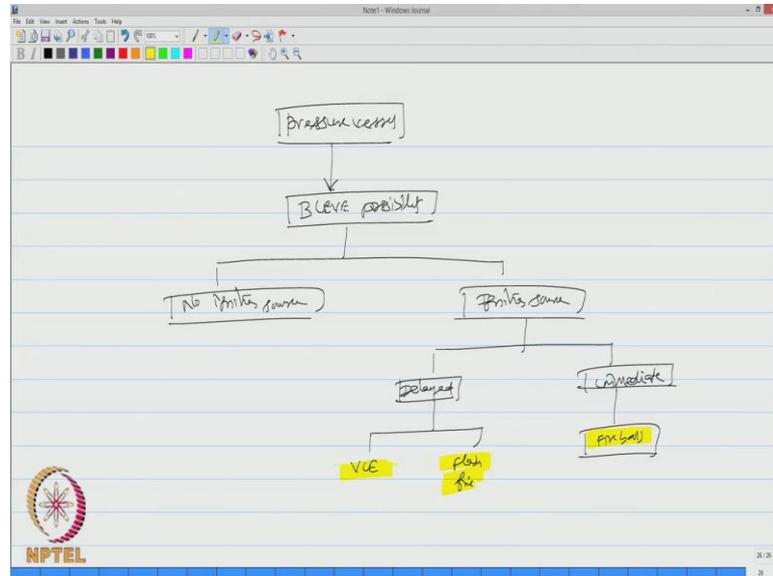
If you look at the flow chart of failure of pressure vessel, we can say pressure vessel will have a BLEVE possibility, we have already seen how and when BLEVE can occur.
