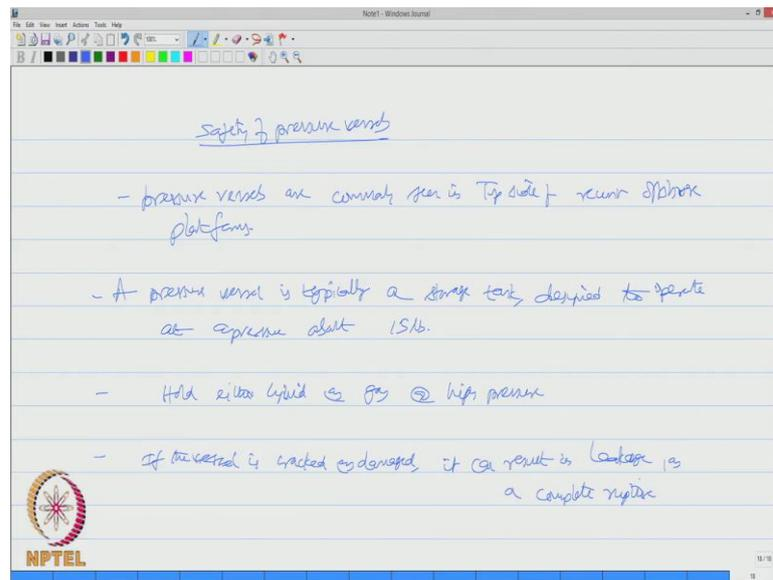
With this background let us extend the discussion for safety of pressure vessels, generally pressure vessels are common in top sides of recent offshore platforms, a pressure vessel is typically a storage tank designed to operate at a high pressure at a pressure about 15 pounds. Generally pressure vessels hold either liquid or gas at high pressure that is why they are called pressure vessels. If the vessel is damaged or cracked it can result in leakage or a complete rupture.
