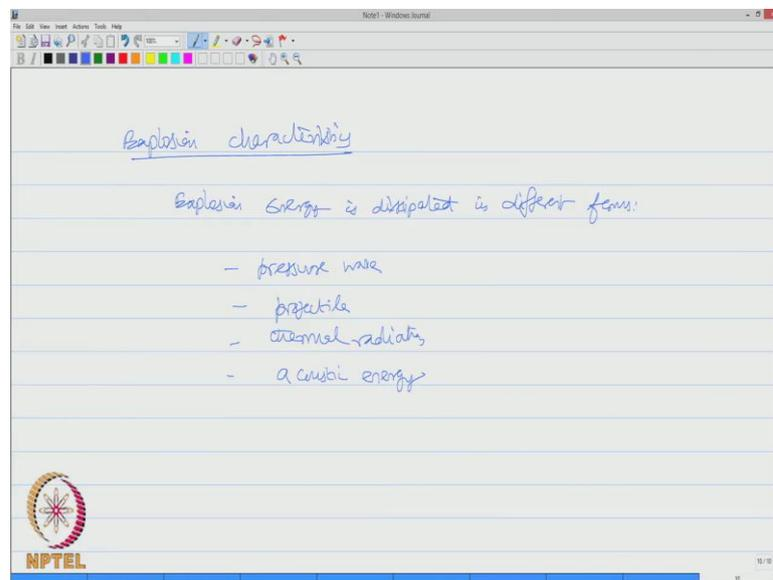
Let us now look into the explosion characteristics; explosion energy is dissipated in different forms, it could be in the form of a pressure wave release, it could be in the relief of a projectile, it could be appearing in the form of a thermal variation and can also be in
