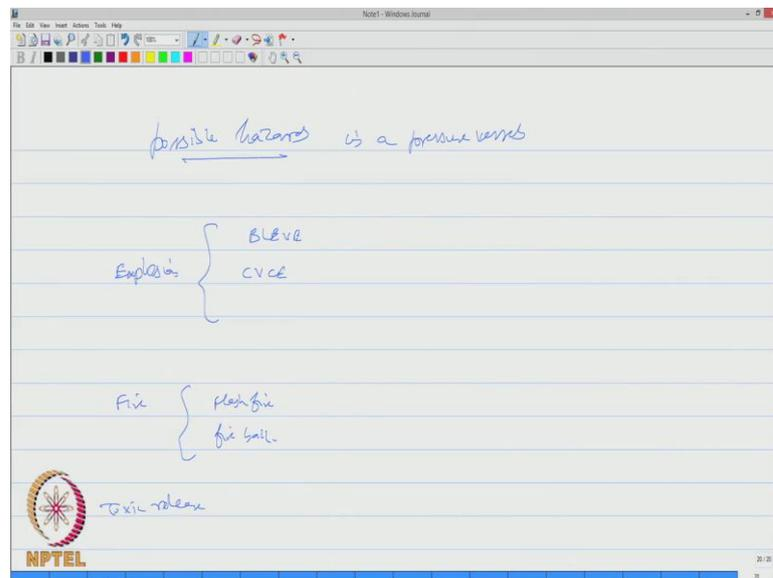
Let us then open a question called what are the possible hazards in a pressure vessel? Because pressure vessels are inherent part of toxic platforms, which are like semi submersibles, drill ships etcetera.
