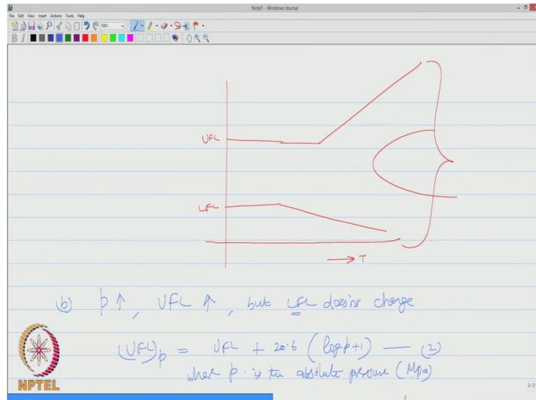
So, this is upper flammable this is lower flammable limit therefore, is may auto ignition therefore, I can say the flammable region increases with increase in temperature as far as pressure is concerned pressure when the pressure increases upper flammable limit increases, but lower flammable unit does not change.
