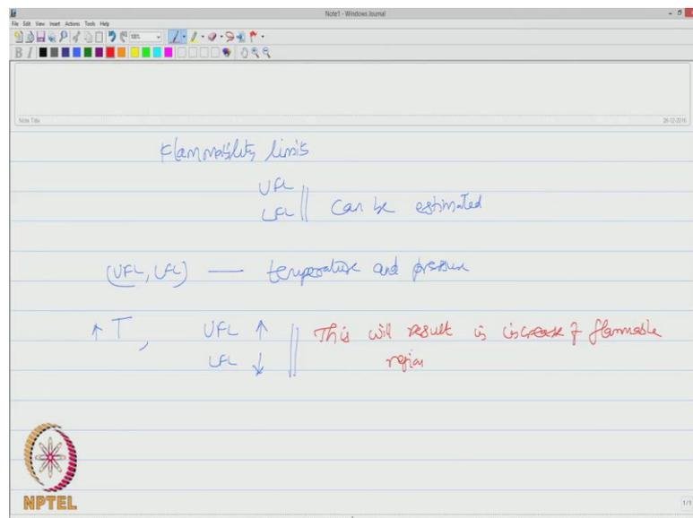
We already said that flammability limits can be experimentally determined using open cup method and the flammability constants  $a$ ,  $b$ ,  $c$  can be evaluated based on which upper flammable limit and lower flammable limit of a mixture can be estimated.
