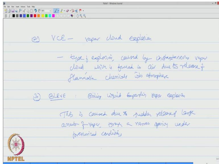
The second one is called VCE, which is vapor cloud explosion. This is a type of explosion caused by instantaneous vapor cloud, which is formed in air due to release of flammable chemicals into atmosphere.
