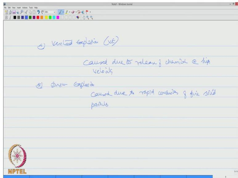
The forth one is vented explosion which is VE; this is caused due to release of chemical at high velocity. The next variety is what we call dust explosion; this is caused due to rapid combustion of fine solid particles.
