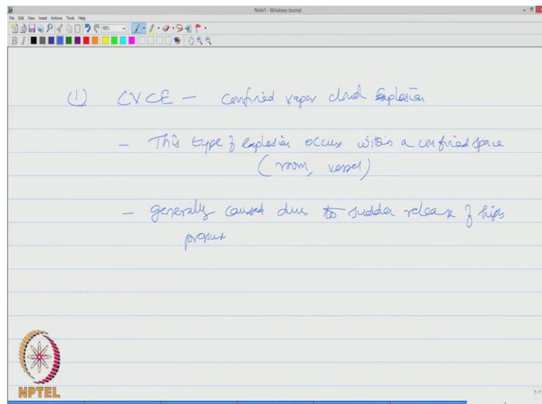
This type of explosion occurs within a confined space, it can happen inside a room, it can happen inside a pressure vessel etcetera.
