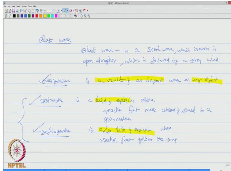
What is a blast wave? Blast wave is essentially a shock wave, which travels in open atmosphere which is generally followed by a strong wind. Over pressure is actually a result of an input wave causing an impact there is an impact wave on any object that is what we call as over pressure. Over pressure essentially is a result of any impact wave on any object.
