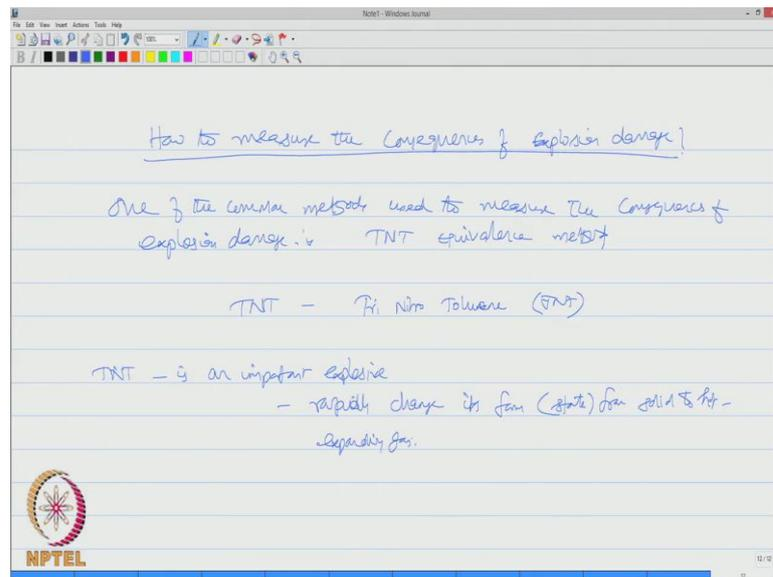
Because that is very necessary in risk assessment; one of the common methods used to measure the consequences of explosion damage is TNT equivalence method. So, TNT is Tri Nitro Toluene; TNT is an important explosive which can rapidly change, which can rapidly change its form or state from solid to hot expanding gas.
