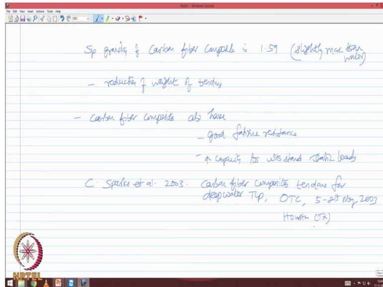
The specific gravity carbon fiber is about 1.59, which is slightly more than water. This enables reduction of weight of tendons; the carbon fiber composites also have good fatigue resistance and high capacity to withstand static loads. More information can be seen from recent studies conducted by C Sparks et al 2003; carbon fiber composites tendons for deep water TLP, offshore technology conference 5-8th may 2003 Hustle.
