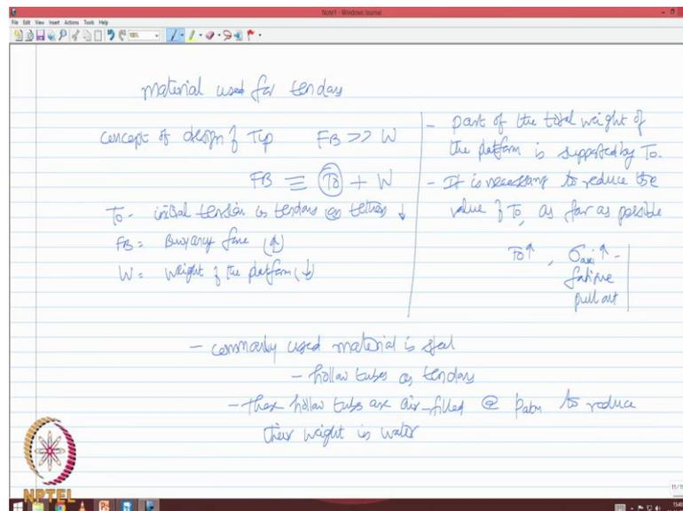
To answer this let us ask the first question, what would be the concept of design of TLP? The conceptual design of TLP is buoyancy should exceed many time by weight. In fact, buoyancy and weight should be equated by initial tension in the tethers. Buoyancy force
