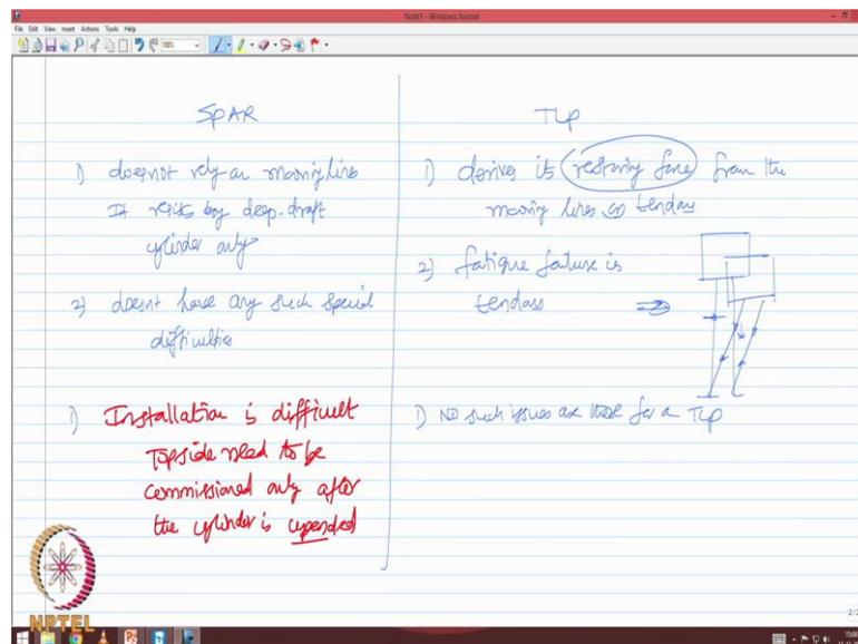
Now, let see why such a decretory difference as been made in the conceptual form of the spare platform compare to TLP. The foremost difference between TLP and spar TLP derives is restoring force from the mooring lines or otherwise called as tendons.
