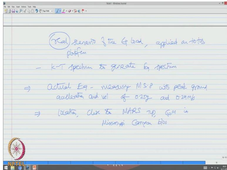
So, one will be interested to know what is the real scenario of the earthquake load applied onto this platform. So, one can actually use the K-T Kanai Tajimi power spectrum to generate the earthquake loads earthquake spectrum.
