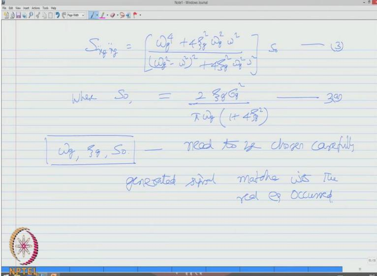
$$S_{\ddot{x}_g \ddot{x}_g} = \left[ \frac{\omega_g^4 + 4\zeta_g^2 \omega_g^2 \omega^2}{(\omega_g^2 - \omega^2)^2 + 4\zeta_g^2 \omega_g^2 \omega^2} \right] S_0 \quad \text{--- (3)}$$
