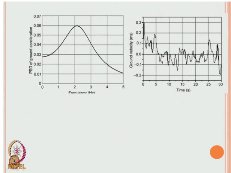
The generated signal typically looks like this; this is the power spectral density of the ground acceleration and the corresponding ground velocity time history, which has been generated using the equations shown to you in the earlier slide.
