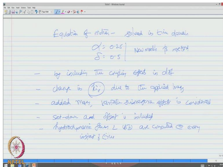
So, equation of motion is actually solved in time domain with alpha as 0.25 and delta as 0.5, we have used a new masks beta method integration scheme to solve this problem. The problem was solved by including the coupling effects in degrees of freedom, by accommodating the change in  $k_{ij}$  due to the applied loads because you know it is a
