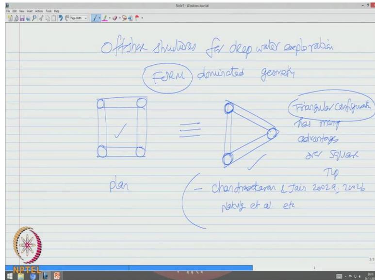
We already said that offshore structures for deep waters are essentially form dominated geometry. So, in that case instead of having a square tension leg platform with all the column members at the intersection that is the plan of the platform, we are looking for an equivalent triangular geometric configuration with only 3 legs.
