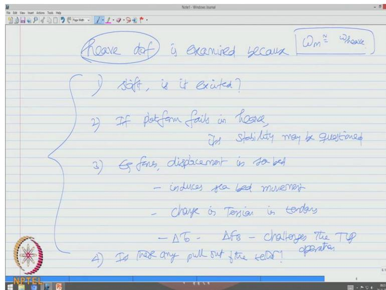
Heave degree of freedom is examined because of the following reasons- the foremost reason is heave being stiff degree is it excited? We want to look into that first. Secondly, if the platform fails in heave, its stability may be questioned; thirdly we are looking for earthquake forces which causes displacement in sea bed and this displacement induces sea bed movement and sea bed movement causes change in tension in tendons, because
