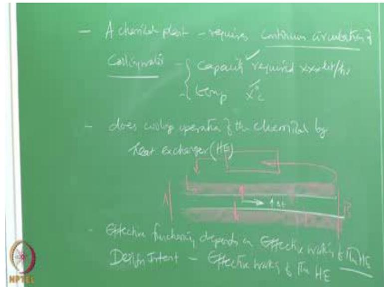
For understanding the deviation in the designed intent consider an example, let us say a chemical plant requires continuous circulation of cooling water the capacity required is xxx car per hour and the temperature at which distribute is apply is x degree Celsius that is a requirement. So, for efficient working of the plant the plant requires the continuous circulation of cooling water at this capacity per hour at this temperature that is a condition working condition.
