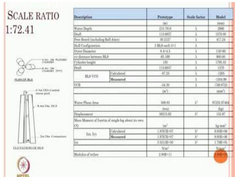
And of course, the ratio was still bigger it made 1 is to 72.41 slightly the model is slightly bigger compared to the earlier one and the BLS was stiff under two points for rigid connectivity between the three units of each leg and of course, you have got positive buoyant system which shows that the system will remain stable.
