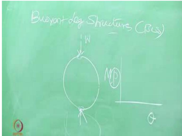
But if you allow the ball joints in my design to happen like this, the ball joint will have terrible rotations in terms of larger rotation in terms of even for a small moment which can be caused either be displacement of the bottom is respect to top or by the wave action or wind action etcetera.
