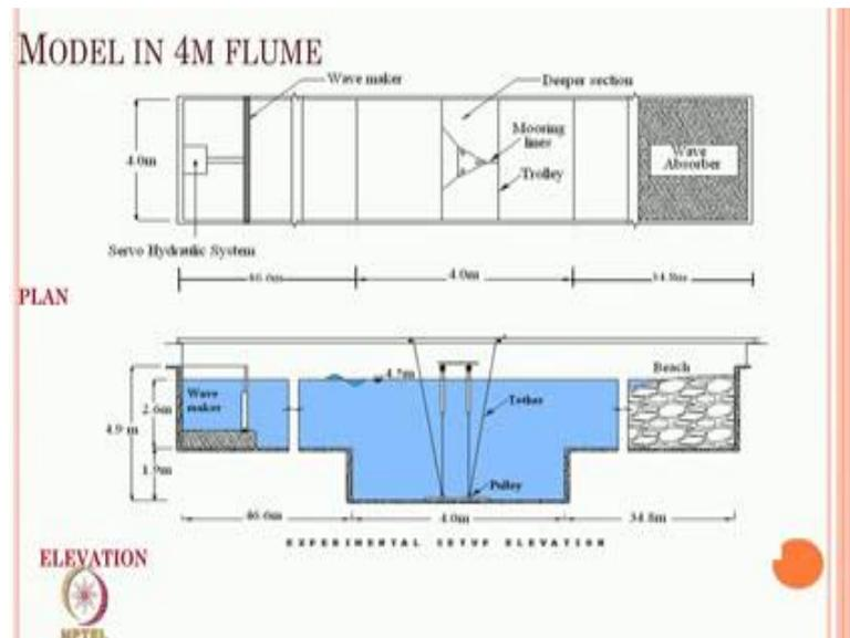
So, the 4 meter flume has got a test bed which is about 4 meter deep at one specific location. So, one can generate a wave using a the wave maker and we have got the depth of the our 4.9 meters at the specific location there is a template at the bottom one can anchor them this is what we called as a (Refer Time: 25:53) arrangement where the tethers are drawn through the pulley and they have been tension at the top it is called top tension risers systems.
