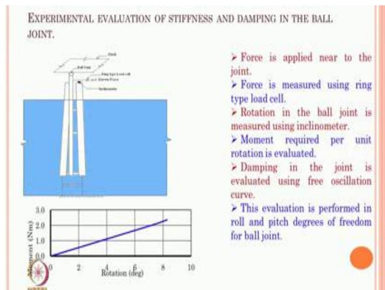
This plot will show you what is the moment rotation characteristic of the ball joint which is more or less linear for a given (Refer Time: 32:34), the force is applied near to the joint force is measured using ring type load cell as you see in the set up here. Then the
