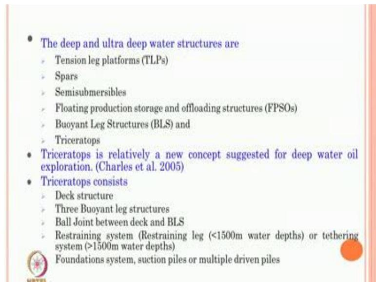
Triceratops was relatively a new concept introduced by Charles et al in 2005 which concerns a deck structure, 3 buoyant leg structures and a ball joint connecting between the deck and BLS. So, BLS and deck were isolated by a special arrangement which is nothing, but a ball joint the restraining system was of course, was similar to the TLP and
