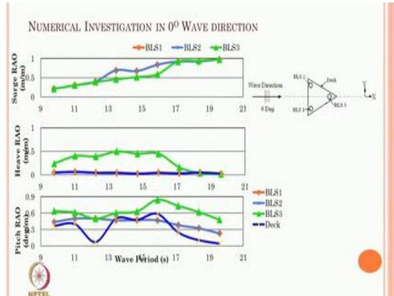
However if you look at the heave degree in terms of earlier for 0 degree, 90 degree etcetera there as mean a complete transformation of a heave motion of the BLS with the deck completely at all the degrees of freedom.
