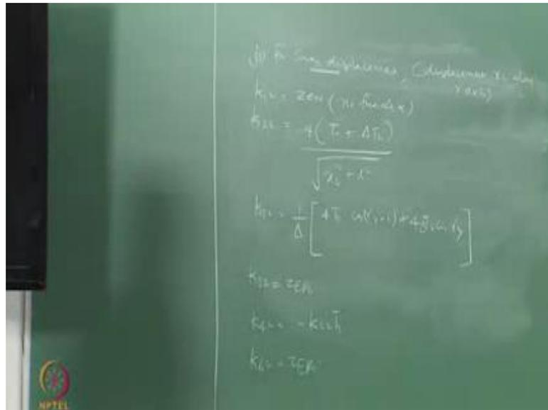
So, for sway displacement - that is displacement along y axis. So, same figure holds good except that I will change the nomenclature slightly I can rewrite the equations readily. So, I will get  $k_{22}$ ,  $k_{12}$  will be 0 because no force along x because of displacement caused along y. Force is already acting along x there is no movement along x because of displacement caused along y because we have to keep all other degrees restrained that is the derivation fundamental in stiffness matrix.
