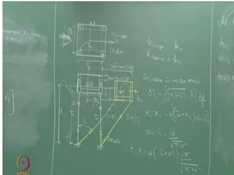
So, if I give displacement along y then I have to draw a view from this direction. So, the right hand side will be to, I am drawing from here - left hand side is going to be 1, right hand is going to be simply 2 and I can say this is x 2, I get the same equation back again only thing is I will change the nomenclature slightly for a sway motion which I am doing it here.
