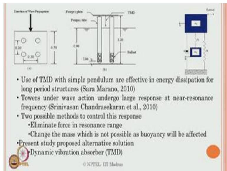
This is actually the physical model which has been done at IIT, Madras. These are the dimensional of the scaled model that is we say system which is shown on the right hand side and this got very good references of Sara Marano which I showed in the last class also. We have also published 1 paper on the same idea on 2010 which I am referring from results. So, the present study actually proposes alternate solution in terms of tuned mass dampers.
