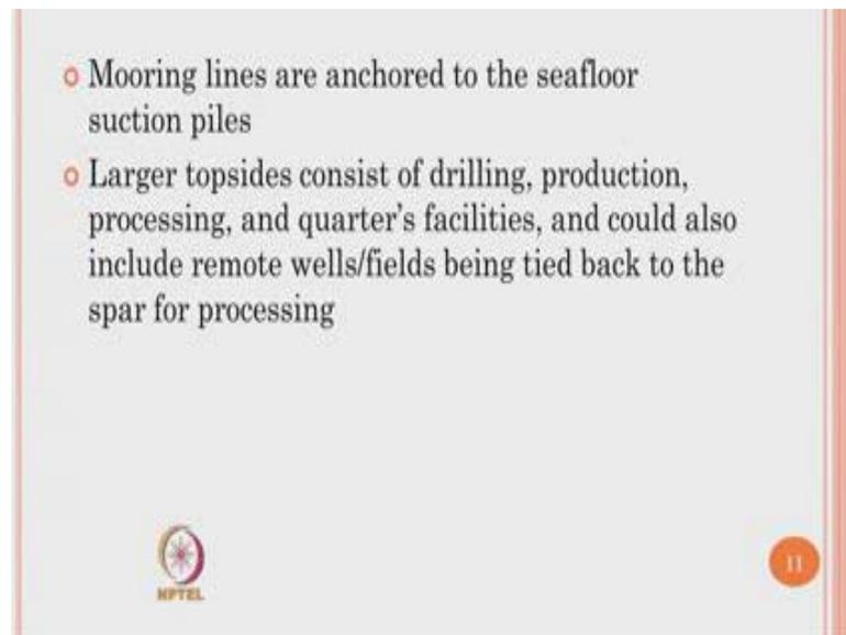
The mooring lines are anchored to the seafloor using piles, which is a suction type pile. Larger top side consist of drilling, production, processing, living quarters, and go also include remote well fields being tied back to the spar for processing.
