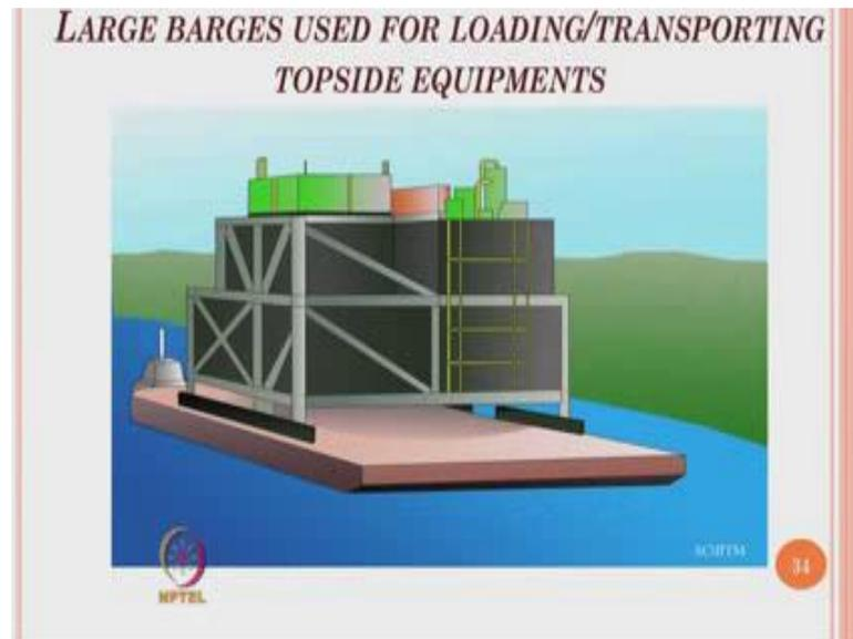
Large barges are also used for loading transporting top side equipments, because you know modular construction is enabled in offshore platform design.
