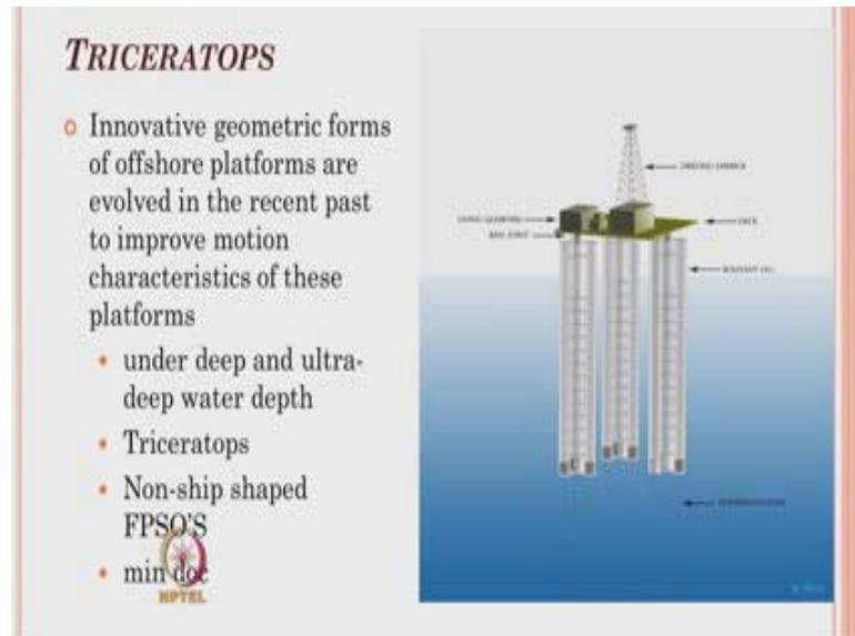
The second verity of structure what you see here which is new generation platform is offshore triceratops. The word triceratops indicates there are three pairs of buoyant leg systems. These are buoyant legs which are not interconnected, which are of course anchored to the sea belt using tethers or tendence as in the case of a TLP.
