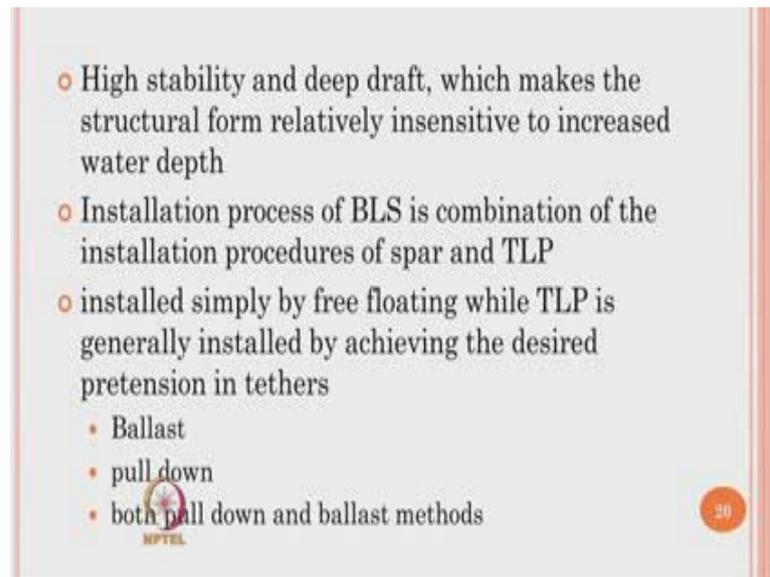
High stability and deep draft makes these platforms insensitive for increase water depth. Installation process of BLS is a combination of installation procedure of spar and TLP. They install simply by free floating, while TLP is generally installed by achieving the desired pretension in tethers either by ballasting or pulling down or both pull down of tethers and ballast methods.
