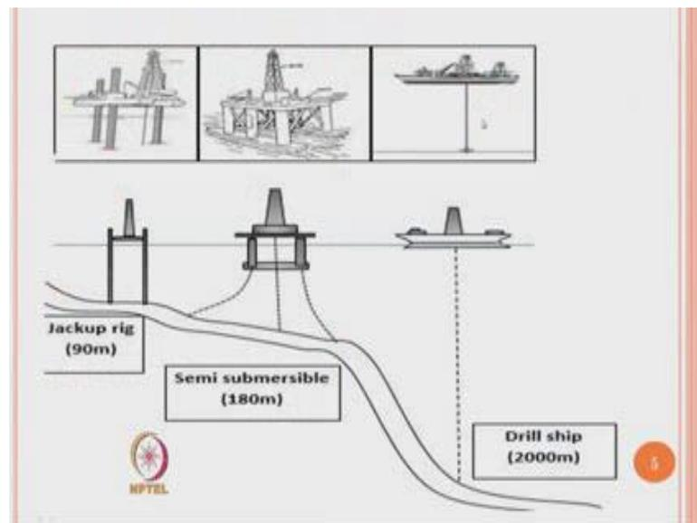
This figure shows you the conception understanding of what kind platform can be deployed floating type can be deployed at different water depths up to 90 or save 100 meters one can go for jack up rigs beyond 100 meters one is comfortable with semi submersible up to about 200 meters and beyond 200 or 250 meters prefer to take a drill ship which can also be capable of exploratory drilling up to depth of as deep as 2000 meters.
