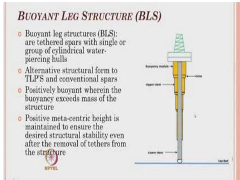
Top on the list in the new generation platform is Buoyant Leg Structure, abbreviated briefly as BLS. A typical tower or stem is connected to the sea bed using a spect scan or a universal joint similar to that of previous kind of an offshore platform. Now the interesting part of this particular type of platform is that there are different buoyancy modules attached to the central tower at different locations so that the buoyancy can be adjusted depending upon sea state.
