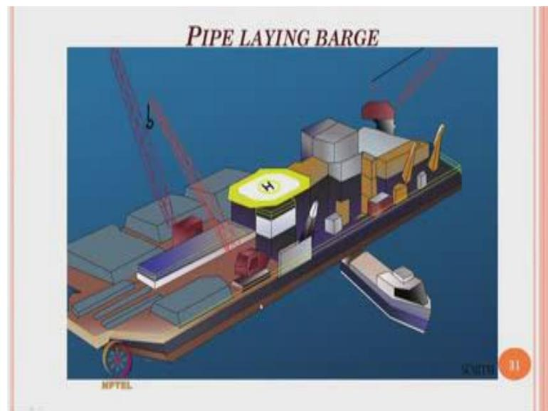
Pipe laying barge is another kind of large floating vessel which essentially used for lying of pipes. Pipes can be used for transporting oil from offshore to onshore locations.
