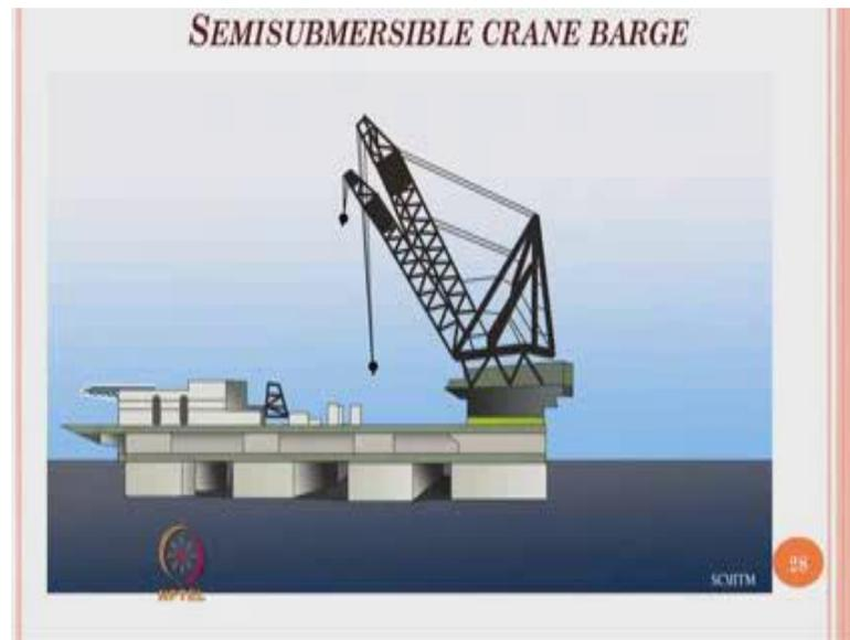
The photograph what you see here is semisubmersible crane barge. Now we can understand very clearly that a platform which is not tankered to the sea bed or connected a sea bed using piles that is semisubmersible needs a crane barge which is used for uploading or transferring oil from one vessel to the another vessel or shuttle tanker.
