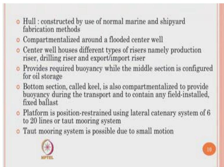
It consists of a hull, which is constructed by a normal marine and shipyard fabrication methods. It is compartmented around the flooded centre well. The centre well houses
