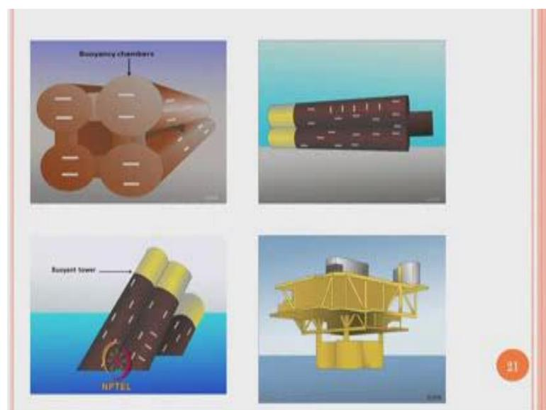
The buoyancy chambers look like this. This is call buoyancy towers, this buoyancy towers are fabricated, interconnected and placed together on a deck mate system as see
