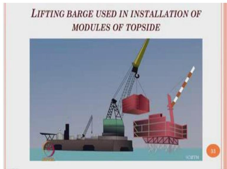
Lifting barge is one of the common facility being used for installation and commissioning during essentially during the top side installation what we call as a (Refer Time: 30:08).
