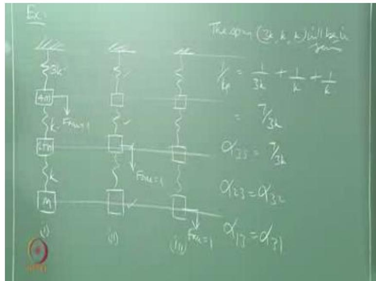
Hence 1 by k equivalent can be 1 by 3 k plus 1 by k plus 1 by k 7 by 3 k therefore, alpha 33 will be 7 by 3 k and alpha 23 will be as same as alpha 32 and alpha 13 will be as same as alpha 31 which we already have here. So, let us enter the alpha matrix here which we want to have which will be a common denominator of 1 by 3 k, so 1 1 1, 1 4 4, 1 4 and 7.
