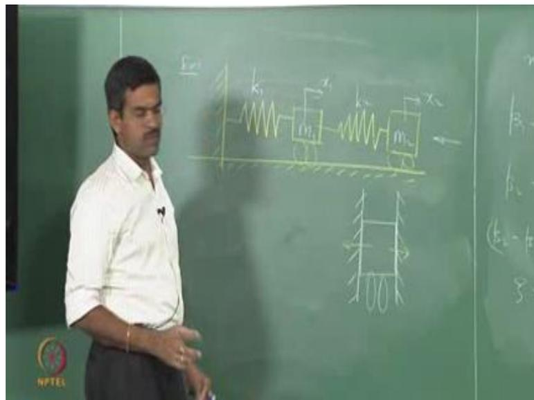
Let us say the system is like, this let us for 2 mass points and to prevent the mass from oscillating in the vertical axis or the vertical plane of the board. I have to put a constraint to this mass, let us the mass rest on roller, why rollers? Rollers will offer no friction to the mass on this plane and roller also prevents mass from oscillating the vertical plane the mass if at all can move only move in this direction.
