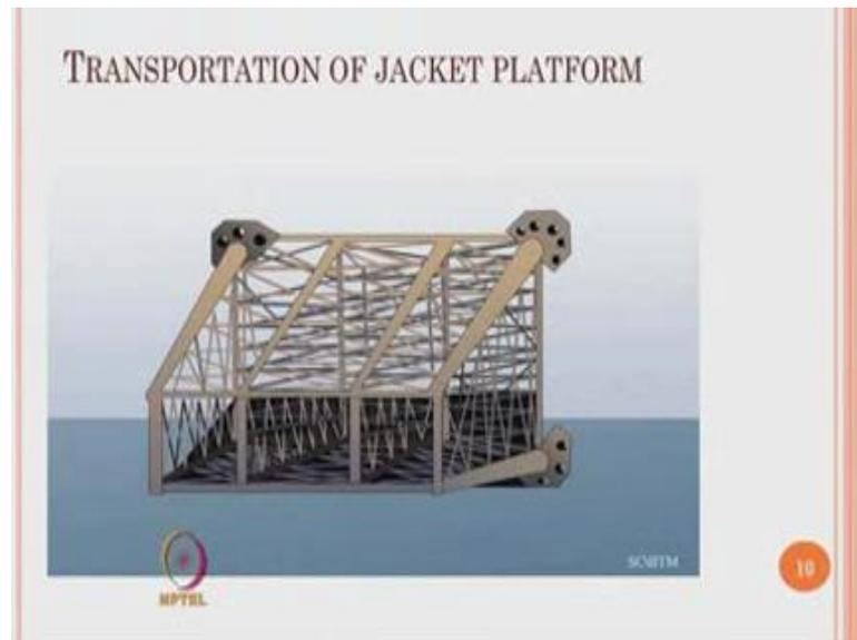
This picture shows you a clear transportation of a jacket platform, you will see that these are the legs which will be anchored to the sea bed through the pile foundation and they are now interconnected with braces and they are also completely battened and lace. So, that the stiff end part of the system is enabling the lateral force distribution along the platform of course, as you saw in the last slide this is now the lying down position, once it is upended this will become vertical.
