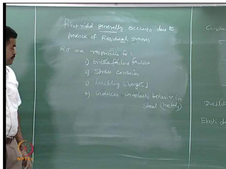
So, residual stresses are responsible for brittle failure fracture, stress corrosion, buckling strength reduction and induces inelastic behavior, please understand this in metals. I am
